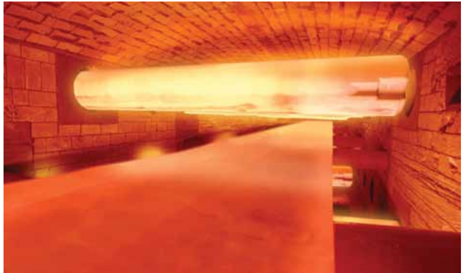
Annealing furnace at ThyssenKrupp Electrical Steel: The new material for electric motors gain their special properties. Source: ThyssenKrupp
