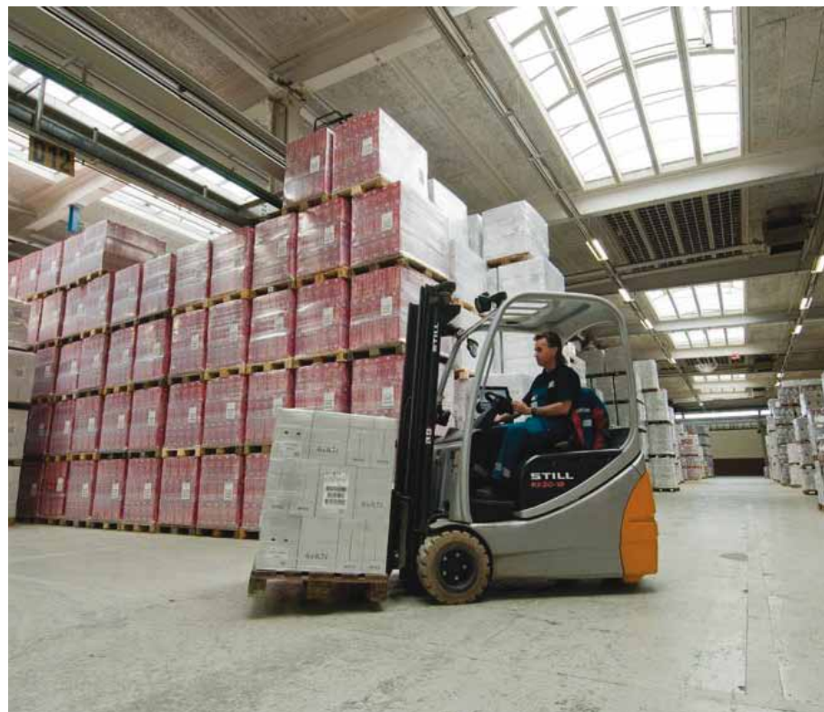
When used as mobile gates, forklifts enable automated information recording. Source: NOSTA
