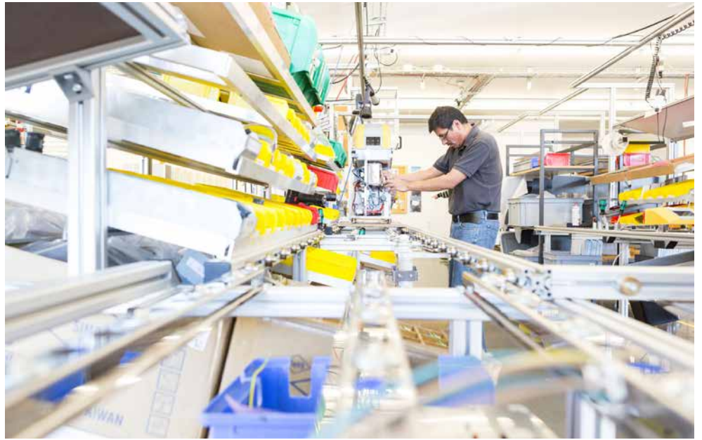
Aequator assembles its fully automatic coffee machines in separate lines per product category in the so-called “one-piece flow”.
